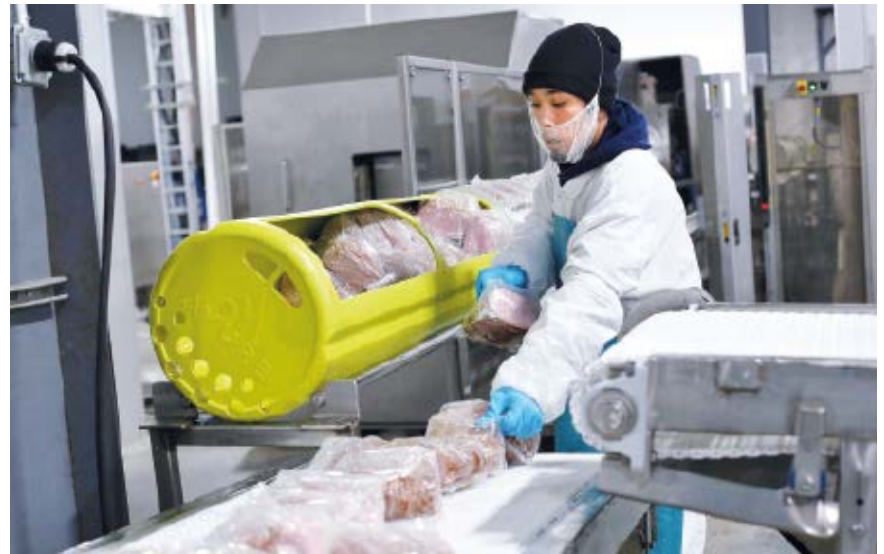
An employee loads meat, sealed in its package, into the HPP canister where it will be subjected to isostatic water pressure.
