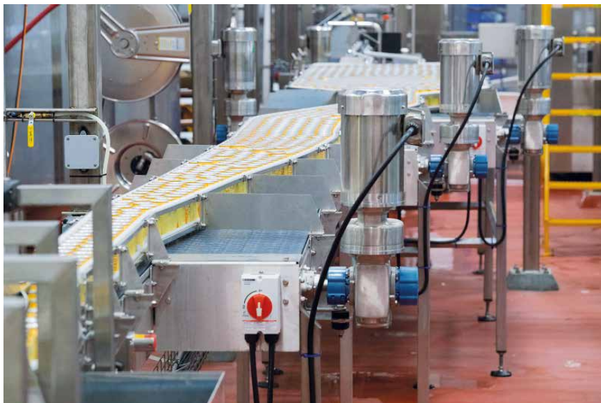
Washdown motors help ensure that Ohio-based MadTree Brewing has a 100-percent dry running conveyor line.
