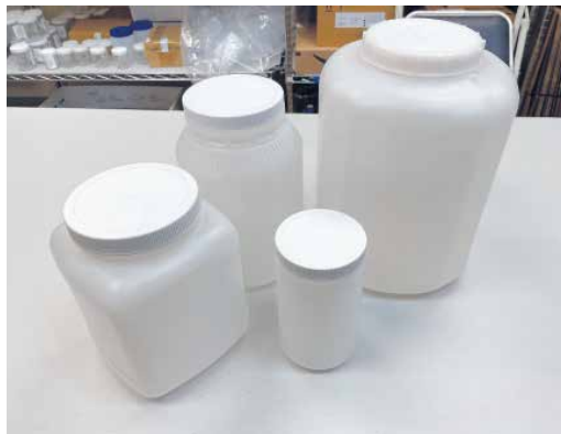
Collect dust samples in a clean, static-free container and follow all laboratory guidelines for storing and shipping your dust.
