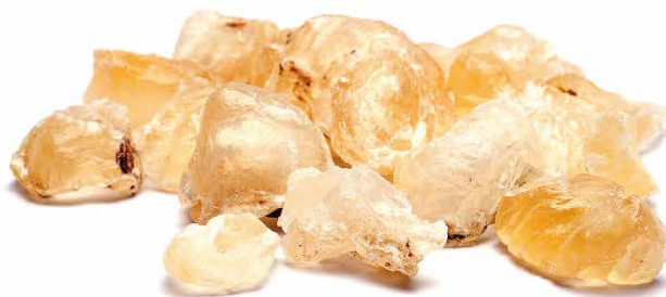
Glycerol esters of rosin are the best known and most commonly used weighting agents in the beverage industry.
