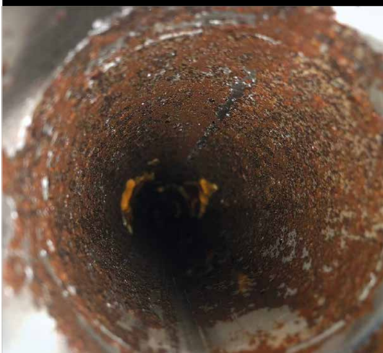
Removal of Maillard reaction fouling in pipes by software-guided power ultrasound. Image 1: Pipe after CIP for 50 minutes without sonication. Image 2: Pipe after CIP with simultaneous sonication for 30 minutes.
