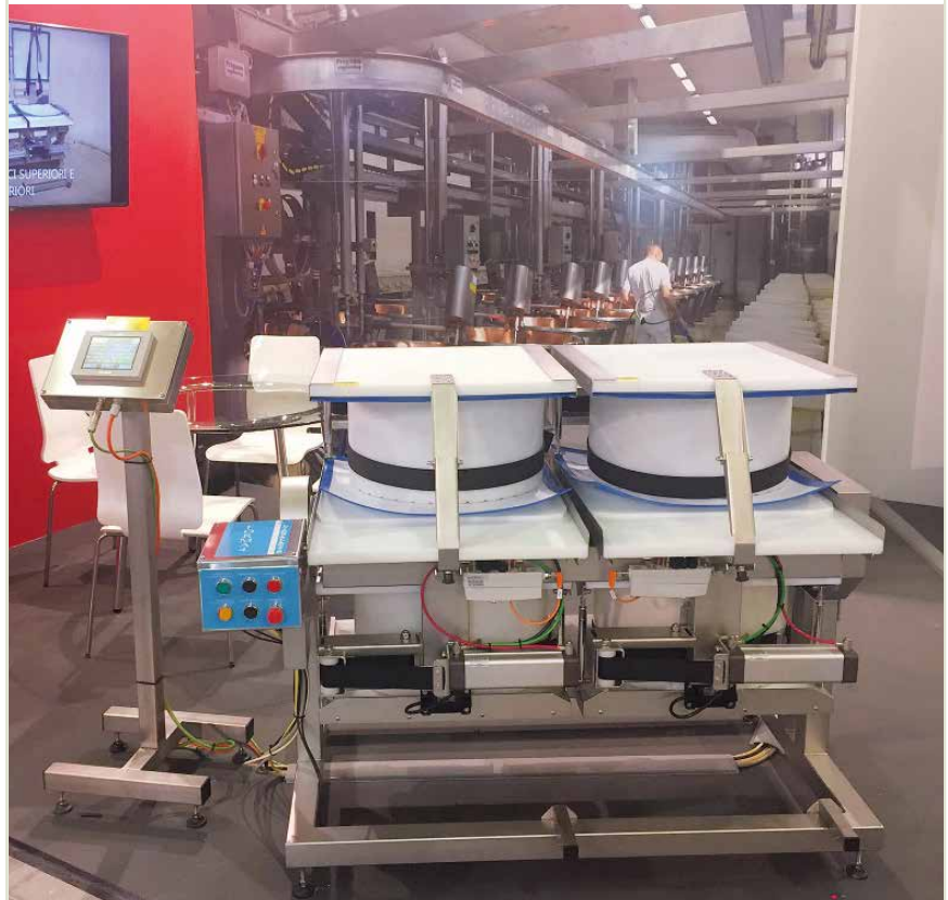
The Emerson AVENTICS washdown CLO3-EV directional control valves (shown left) are installed directly on the cheese-making machine (below), with actuators in decentralized locations, so that compressed air lines are shorter with no dead volumes or pressure losses, thereby reducing air consumption.
