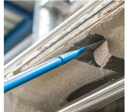
Figure 3: Use scrapers to remove dried or baked on soils, and heavy grease, or confectionary deposits.
