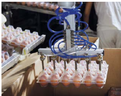
Collaborative robot arms from Universal Robots belong to an emerging new class of industrial robotics that can operate outside of safety enclosures alongside employees.
