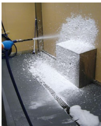
Foaming PAA penetrates sporecoats and provides enhanced residence time of the biocide on target surfaces.
