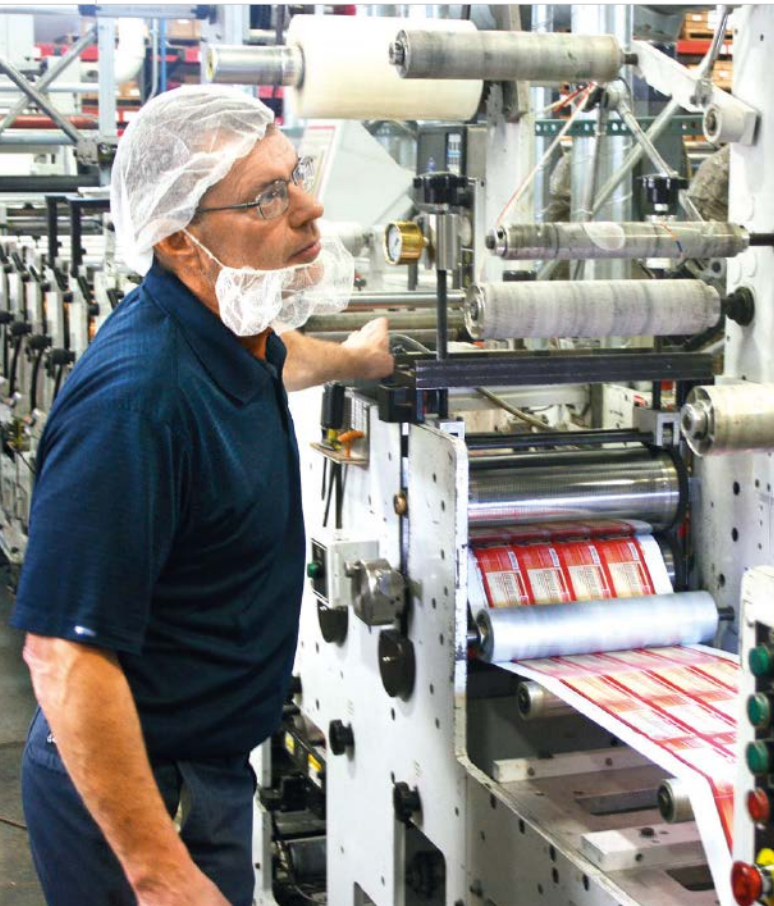
Press operators should wear hair nets, beard masks, and gloves when running food labels.
