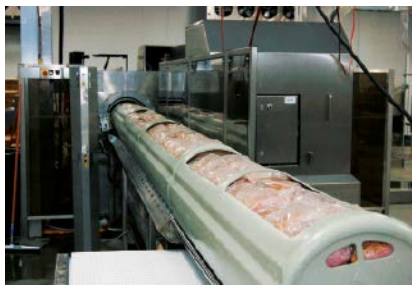
During HPP, products already sealed in their final packages are introduced into a vessel and subjected to a high level of isostatic pressure.
