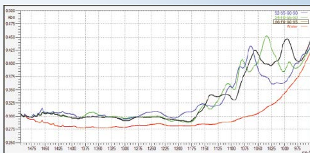
Figure 2: FTIR spectra of 5% aqueous solutions of water (red), fructose (blue), glucose (green), and sucrose (black).
