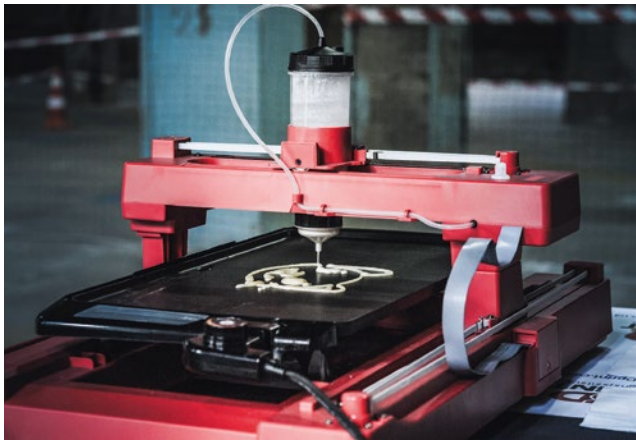
The 3D printing of dough for pancakes.
