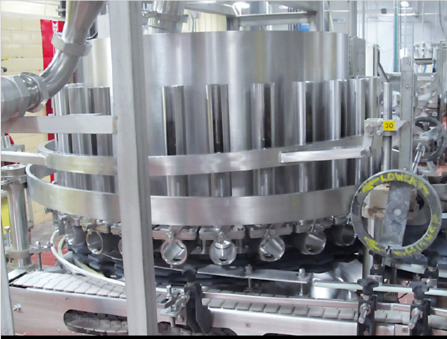
New piston filters come surrounded by a complete guarding package to protect the operations; however, the perimeter guarding must be added to used ones.
