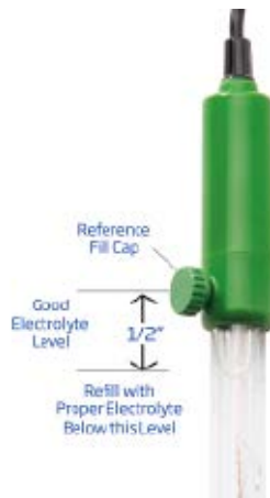
Maintaining electrolyte fill levels helps obtain more stable readings.
