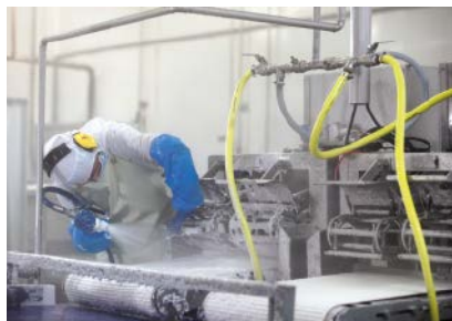
Interroll's drum motor design can be washed down at high pressure and can protect against particles.
