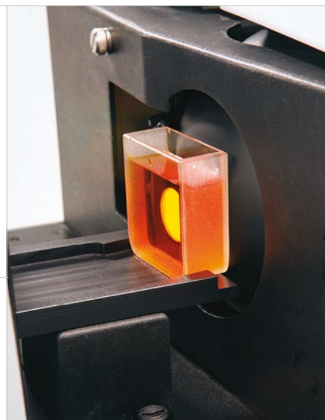
Soft drink sample measured with transmission instrumentation.
