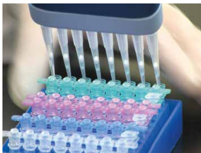
The 3M Molecular Detection System offers a sample preparation process without DNA extraction and purification steps.
