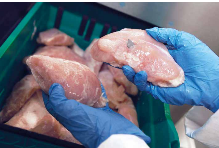
Stainless steel detection signals can be swamped by product effect in wet or salted products.
