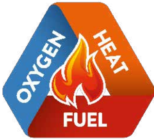
Figure 1. The Fire Triangle. Fires require fuel, oxygen, and heat or ignition.
