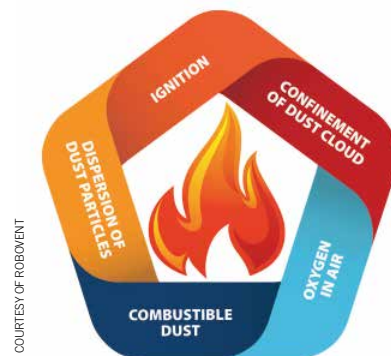
Figure 2. The Explosion Pentagon. A combustible dust explosion requires fuel (combustible dust), oxygen from the air, and an ignition source, PLUS dispersion of the dust in a cloud and confinement of the dust cloud. In the absence of confinement, ignition of a cloud of combustible dust will result in a flash fire.
