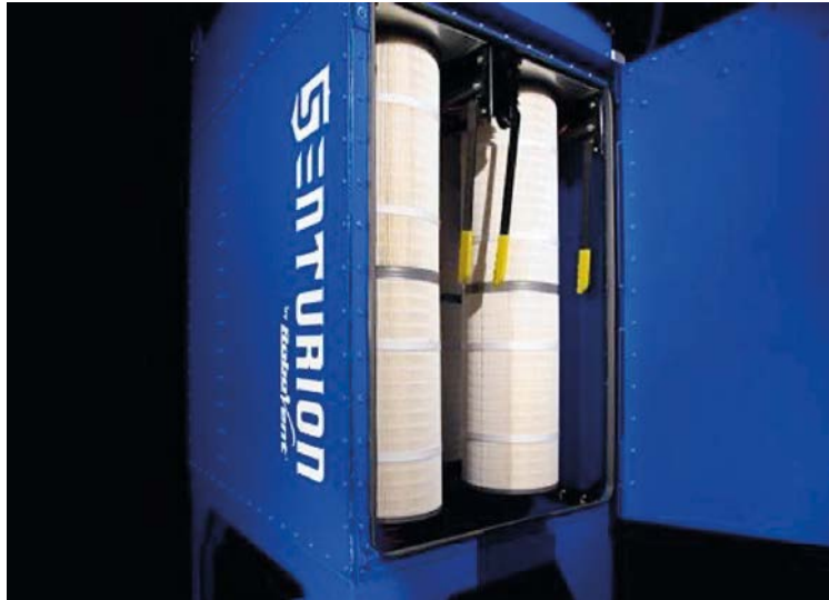
A cartridge dust collector pulls dirty air through a filter chamber and returns clean air to the facility.
