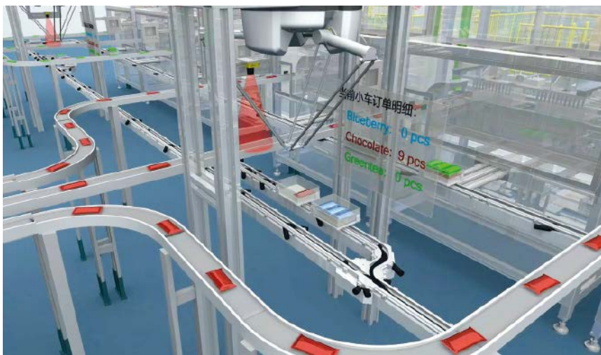
Frozen food line simulation featuring independent cart technology.
