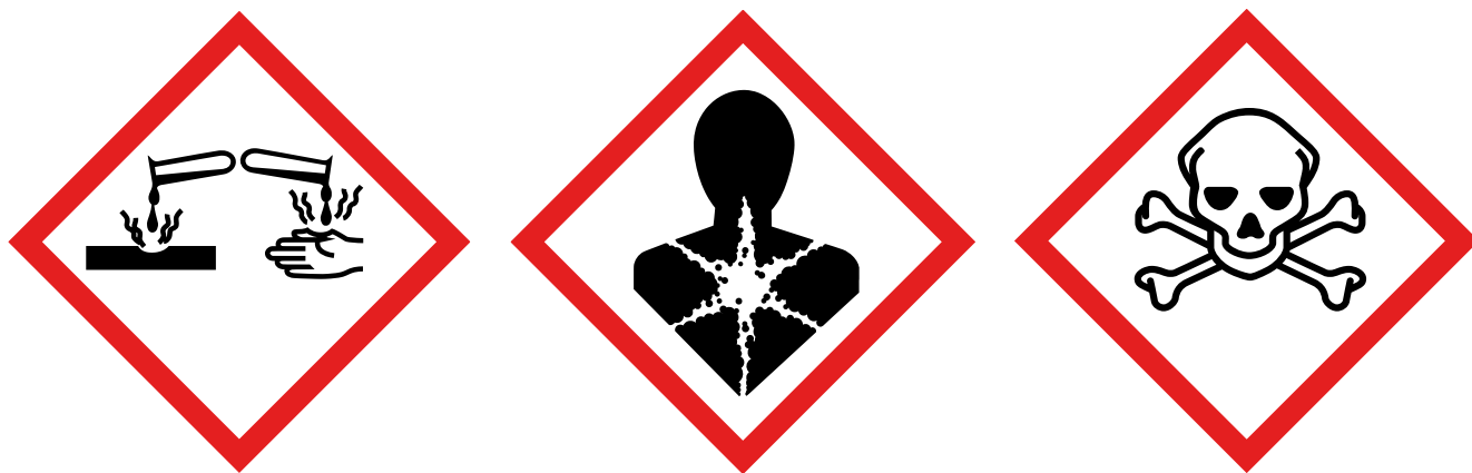
Figure 1. Pictograms warning of (from left to right) corrosion, health hazard and acute toxicity (fatal or toxic).
