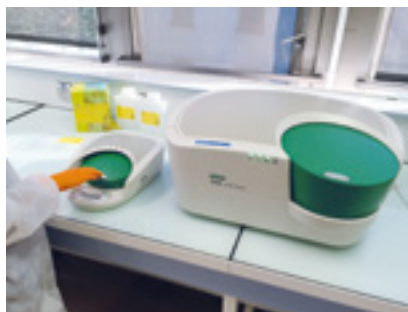
The QX200 Droplet Digital PCR System from Bio-Rad Laboratories is intended to reduce the number of false positive samples.
