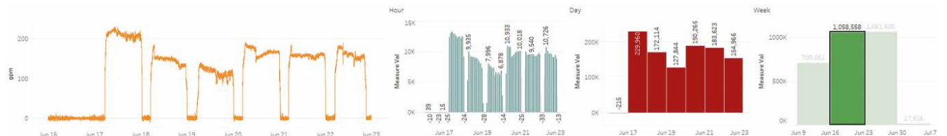
Figure 3: Water use data demonstrating flow rate and hourly, daily, and weekly volume aggregation. This data shows that while similar water needs were steady throughout the week during the production time period, volume rates changed dramatically, revealing the potential for water optimization.
